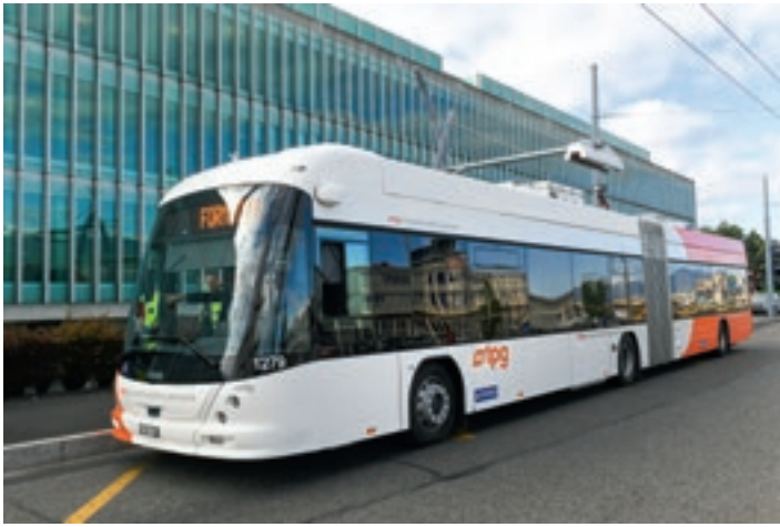
TOSA electric bus uses flash-charging technology.
