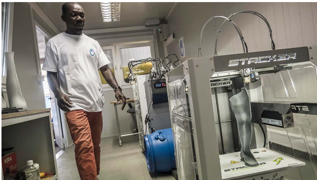
Togo, an International Handicap technician, prepares a 3D-printed orthopaedic support in Lomé.
